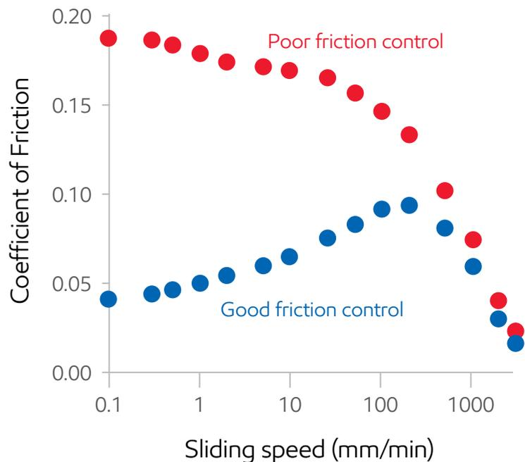
Test conditions: Slideway Friction Test Rig (University of Darmstadt) - dynamic friction, metal-to-metal
