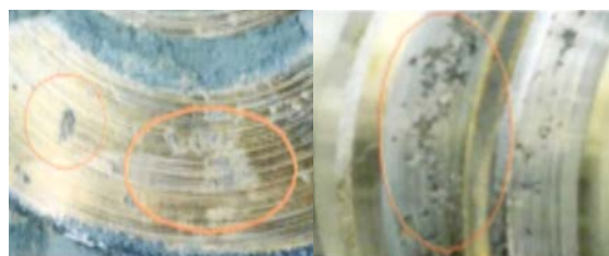
After 30,000 rotations with the mineral oil as the lubricant, dispersed pitting on the wheel and worm gear surface can be seen.
